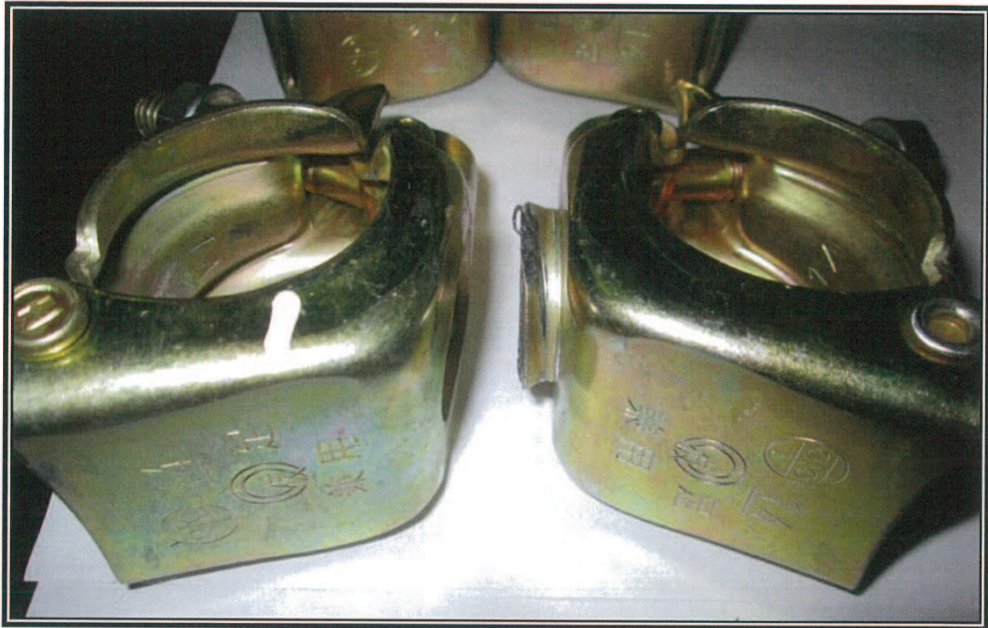
Photograph 3: Shows failure mode of the tested samples Set 1
