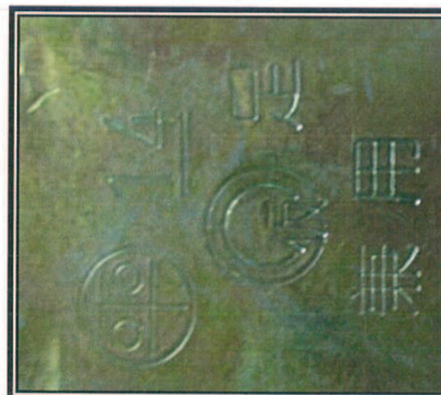
Photograph 2: Shows sample marking on the couplers - Closed-up view
