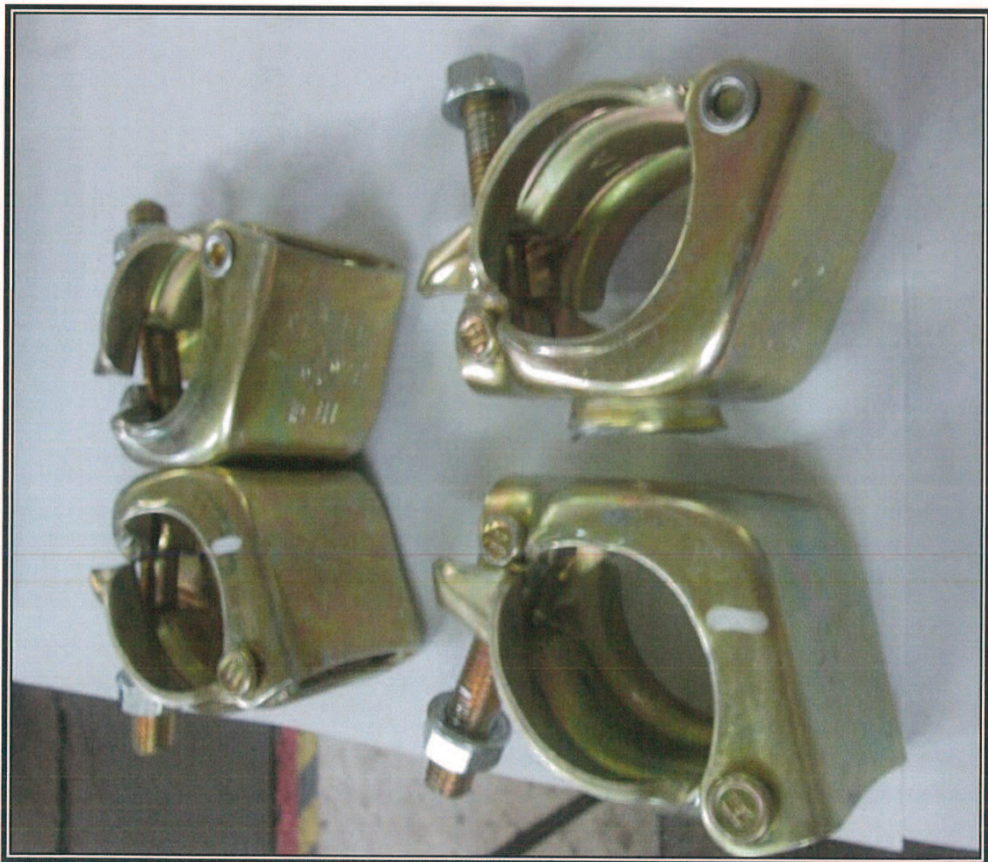
Photograph 4: Shows failure mode of tested sample Set 1
