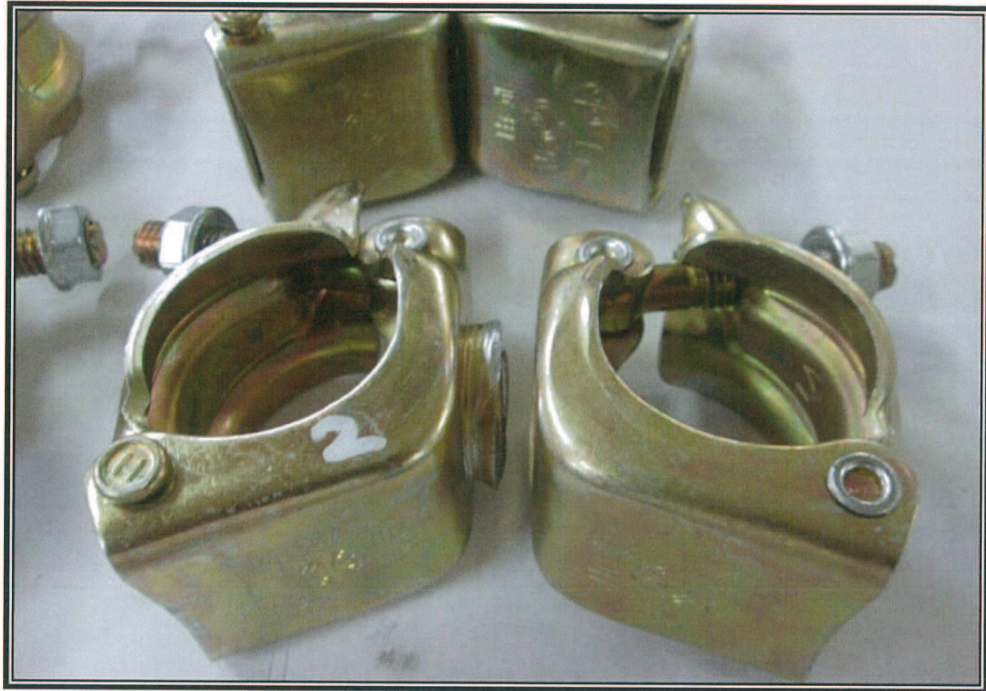
Photograph 5: Shows failure mode of tested sample Set 2
