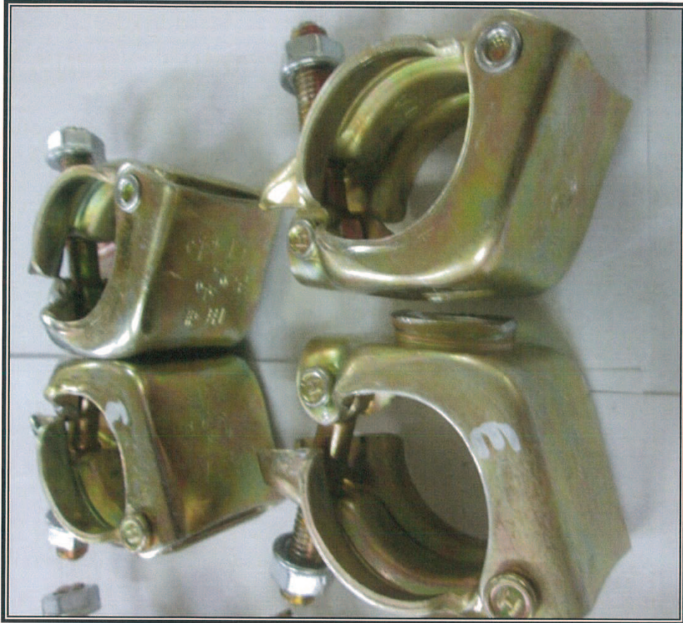
Photograph 7: Shows failure mode of tested sample Set 3
